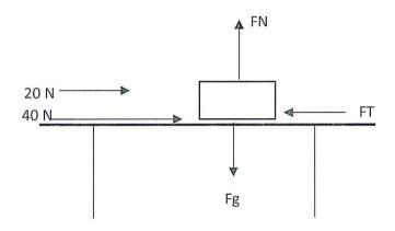
Given that the wooden object is having a force of gravity (Fg) of 20 N and acceleration due to gravity of 10 ms<sup>-2</sup>.
